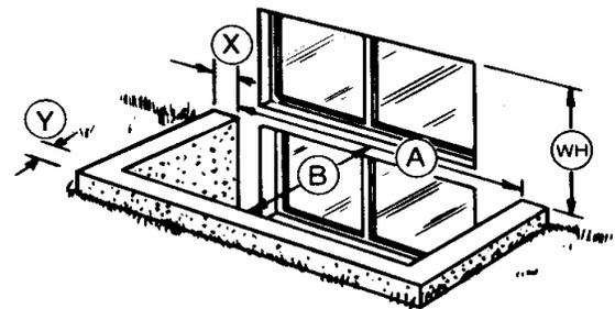
Model 4-R Window Bubble covers rectangular style masonry or wood wells.
